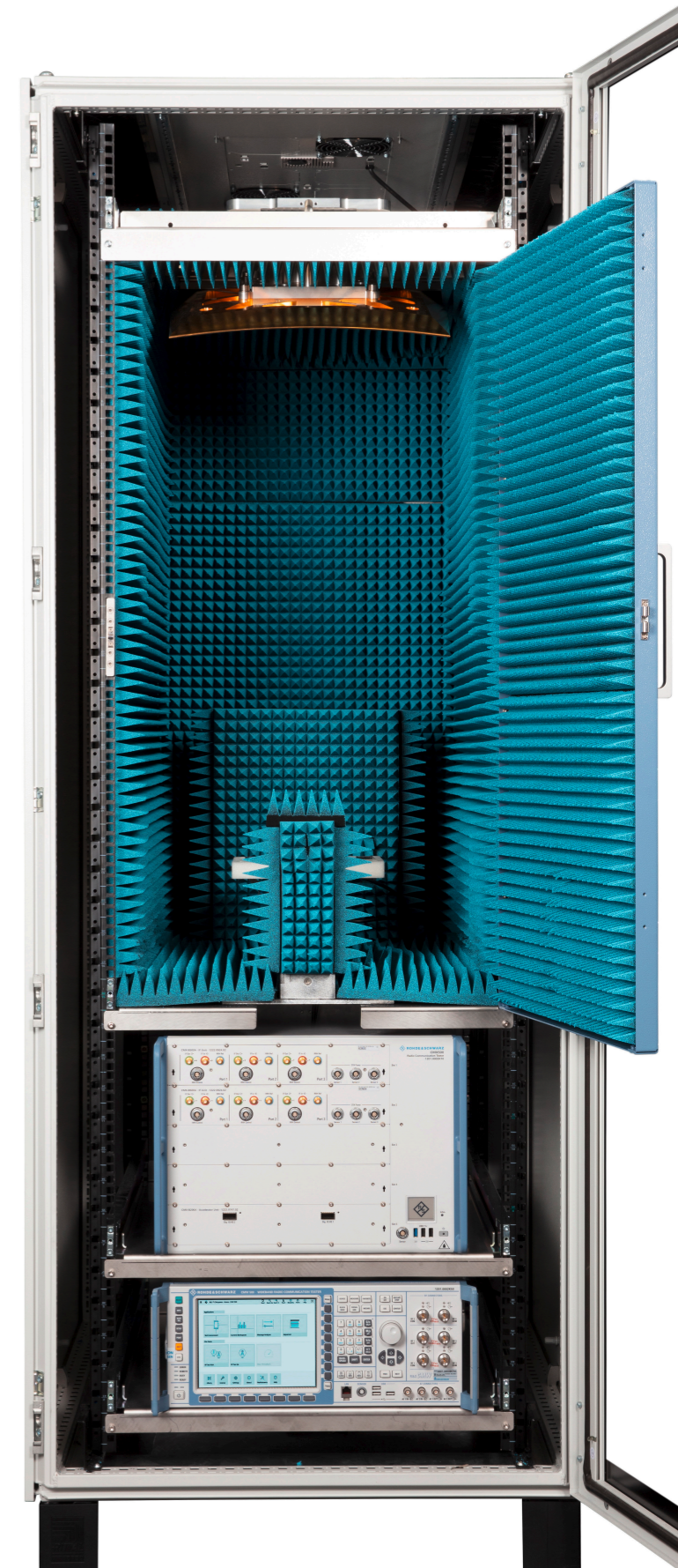
The R&S®ATS800R rack based CATR antenna test system together with the R&S®CMX500, R&S®CMW500, 2 × R&S®CMXHEAD30 and R&S®CMX-RF42 is used for the OTA setup.
