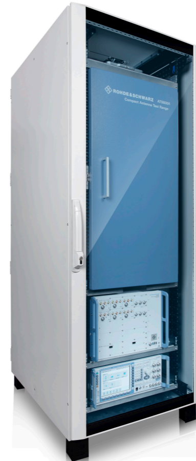
R&S®ATS800R with the R&S®CMX500 and the R&S®CMW500 wideband radio communication tester.
